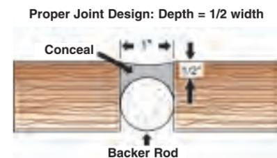
For joints 1" wide or more, the depth should be 3/8" to 1/2". The depth of joints less than 1" wide should be
